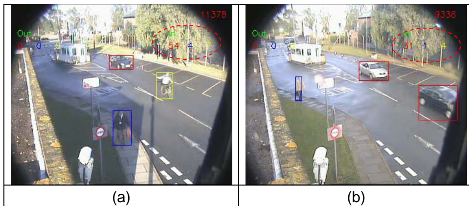
Figure 10: The site's Northgate security camera view and the illustration of classification and counting results: cars in red, pedestrians in blue, cyclists/motorists in yellow blob, respectively; the dashed red ellipsis recording the real-time counts so far.
